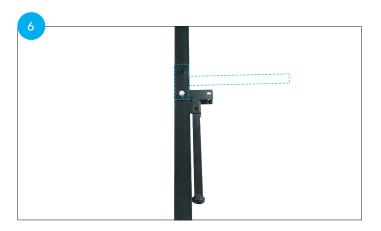
Rotate the middle legs out and align the holes.
