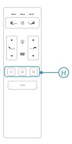
**NOTE:** To restore the preset buttons back to their original factory settings, hold <u>FLAT</u> and <u>ZERO-G®</u> simultaneously for at least 5 seconds. The original presets will be restored.
